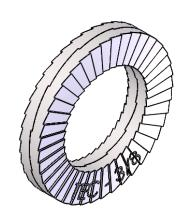
DIMENSIONS ARE IN INCHES TOLERANCES: ANGULAR: MACH ± 1 BEND ±1 I.D. TOLERANCE: ±.008 O.D. TOLERANCE: ±.008 THICKNESS TOLERANCE: ±.01 MTB 2/27/17 DRAWN CHECKED JVK 2/27/17 ENG APPR. INTERPRET GEOMETRIC TOLERANCING PER: MFG APPR. ASME Y14.5M-1994 MATERIAL Q.A. SCM435 OR 4130 STEEL, COMMENTS: HT: THROUGH HARDEN E-mail: info@disc-lock.com 465 HV MIN
